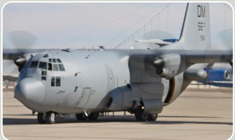
The 55th ECG's flagship EC-130H on the ground at Phoenix-Mesa Gateway Airport. The 55th relocated to Gateway for a week during 2011 when D-M's runway was being resurfaced. Note the wire antenna on the tail and the large aerials protruding from the rear fuselage, both components of the Rivet Fire electronic warfare system. - photo by Joe Copalman.
